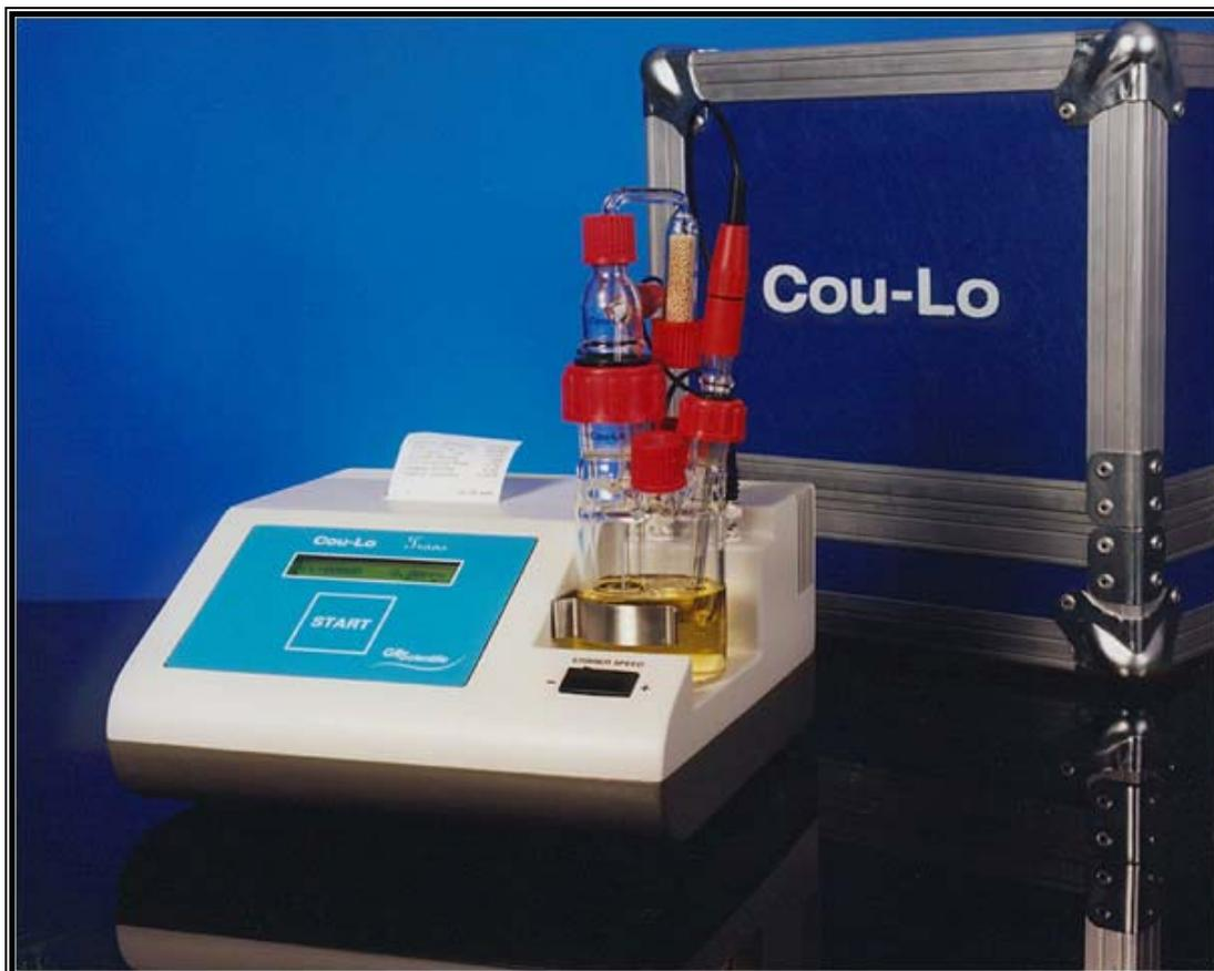
**TITOLATORE COULOMETRICO KARL FISCHER, COMPATTO, PORTATILE, CON AGITATORE INCORPORATO, CONFORME ALLA NORMA BS 60814, RELATIVA ALLA DETERMINAZIONE DELL'UMIDITÀ DELL'OLIO DEI TRASFORMATORI**
